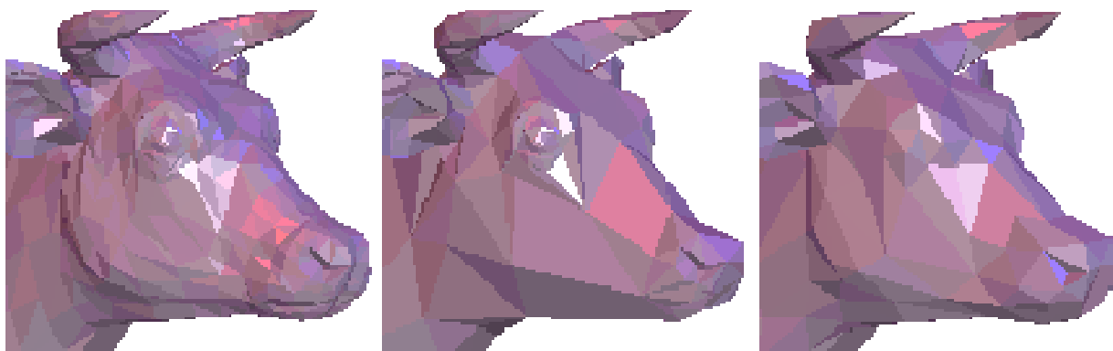
Figure 11: Comparison with QEM. The left model is the original with 5,804 faces. The middle and right models are both simplified to 2,000 faces using our scheme and QEM respectively.
